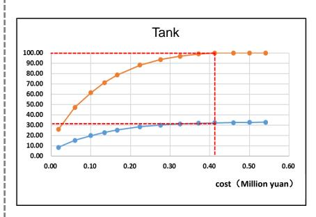
• When the volume of the tank is 2.5m³, the rainwater collection efficiency and percentage of meeting requirement increase as the cost increases, and the growth rate slows down.
