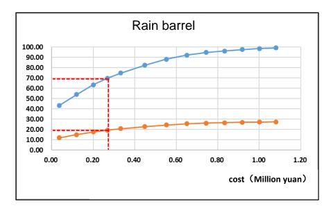
• When the volume of rainwater barrel is 1.5m<sup>3</sup>, the rainwater collection efficiency and percentage of meeting requirement increase as the cost increases, and the growth rate slows down.
