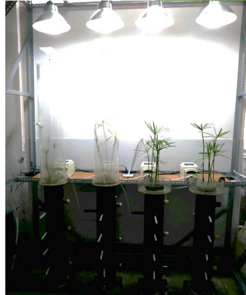
Lab-scale CW for CH 4 emission control
