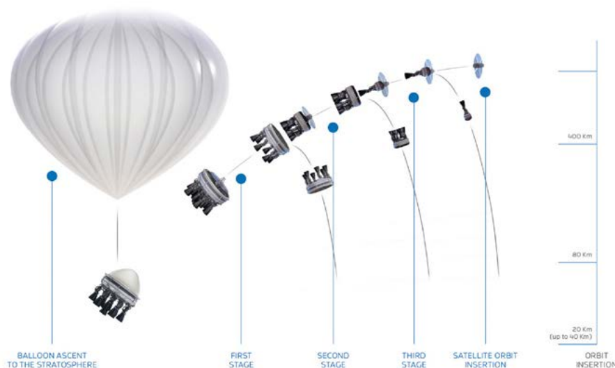
The five phases from balloon-start into the orbit
