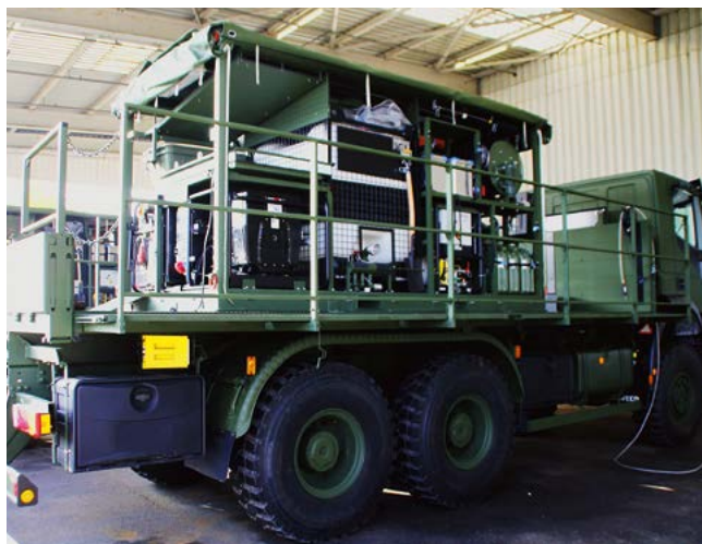
The Decontamination System CDS 1000 – This compact system can decontaminate vehicles, material and persons.
