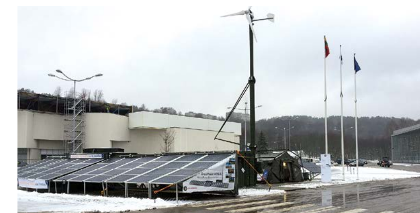
The Hybrid Power Generation and Management System (HPGS) was part of the IESMA 2016 exhibition. This deployable modular system, developed by the German company Pfisterer, was handed over by the ENSEC COE to the Lithuanian Armed Forces in February 2016. The HPGS utilises both, renewable energy sources and conventional fuel, and includes batteries and a management system.
